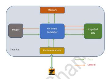
the images to be analysed and the application returns the compressed image ready for transmission to the ground station.
