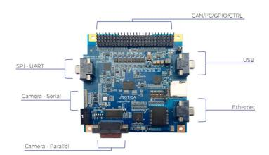
Note 1: Use of these interfaces is not supported by the standard firmware supplied with the CogniSAT-XE1. Contact Ubotica to find out how to utilise these interfaces.
